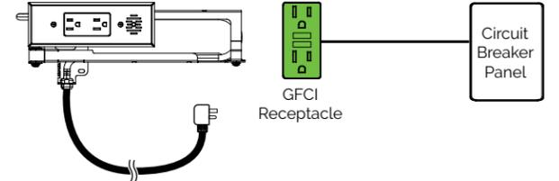
**Option 2 - Wired in a series with a GFCI outlet**
