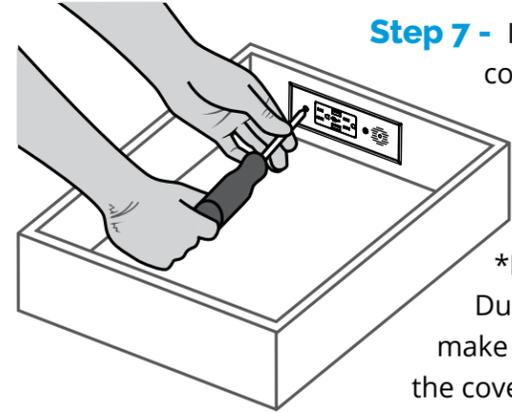
\*For Blade Duo outlets, make sure that the cover plate is installed so that it covers the receptacle box flanges.
